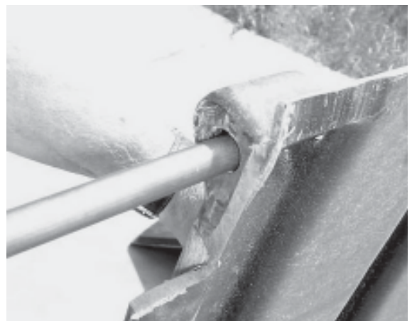
Insert pin through all lid hinge bosses.
